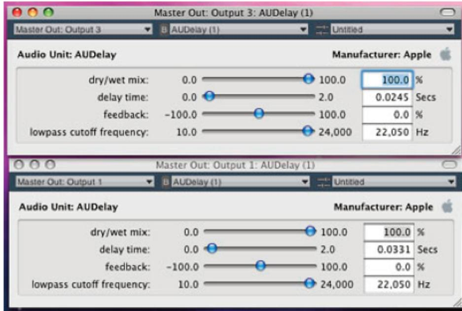
As shown above, AUDelay plug-ins were added as Effects to the signal buses in AuLab on the receiving computer. One signal output bus (stereo output) was delayed by 24.5 milliseconds, and the other 33.1 milliseconds.
