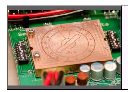
The Seta DAC Buffer uses a unique video - bandwidth amplifier module which is electronically and acoustically isolated as well as kept at a stable operating temperature and environment (constant humidity) by enclosing and sealing in a block machined from a solid piece of oxygen-free high conductivity copper.
