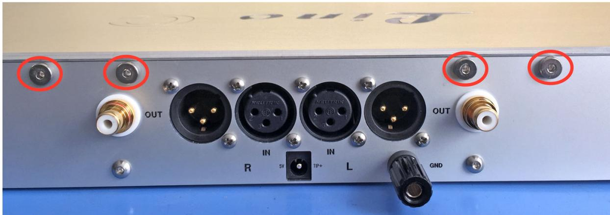
4. Remove the four flat head hex screws (indicated in image above) from the rear panel using the supplied 3/16" hex key.
