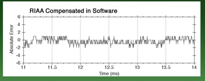
Modulation of RIAA compensated error significantly (24.6 dB) smaller than expected (based on headroom requirement)
